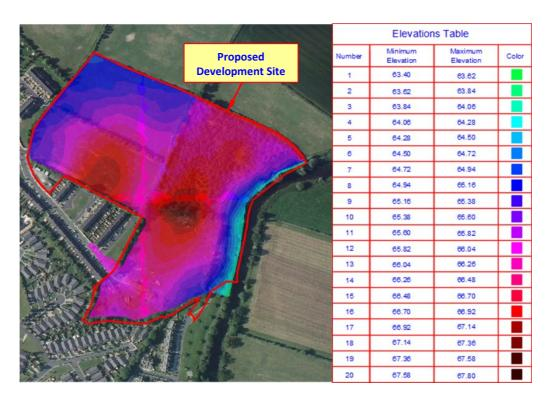
Figure 15 - Topographical Survey Derived DTM
