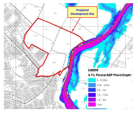
Figure 12 – Eastern CFRAMS 0.1% AEP Fluvial Flood Depth Map
