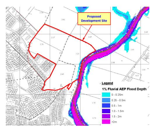
Figure 11 – Eastern CFRAMS 1% AEP Fluvial Flood Depth Map
