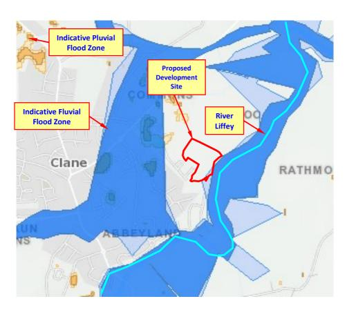
Figure 5 - PFRA Indicative Fluvial Flood Mapping
